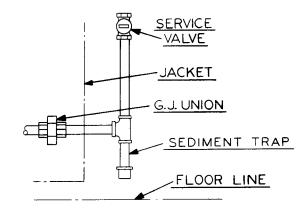
Figure 5.1: Gas Connection to Boiler
